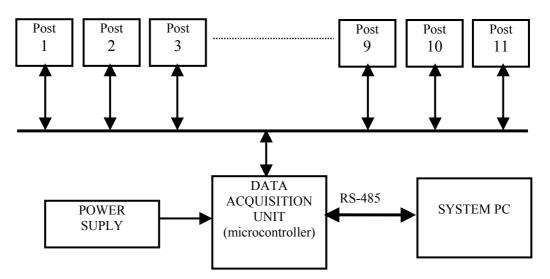
Fig. 1. The block scheme of monitorning system of spark plugs production.
