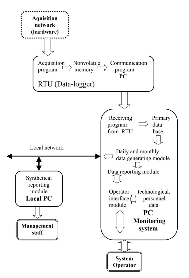
Fig.2. The structure and position of acquisition, monitoring and reporting software modules for spark plugs production.
