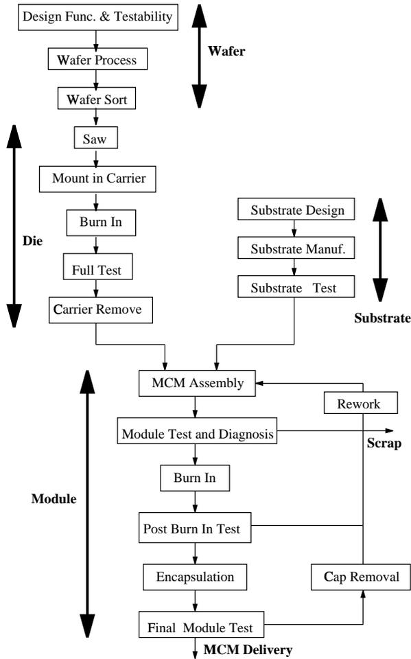
Figure 1: MCM Production and Test Flow
