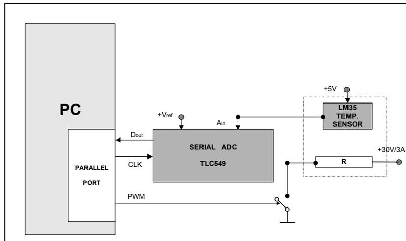
*Figure 1: The schematics of the application*
