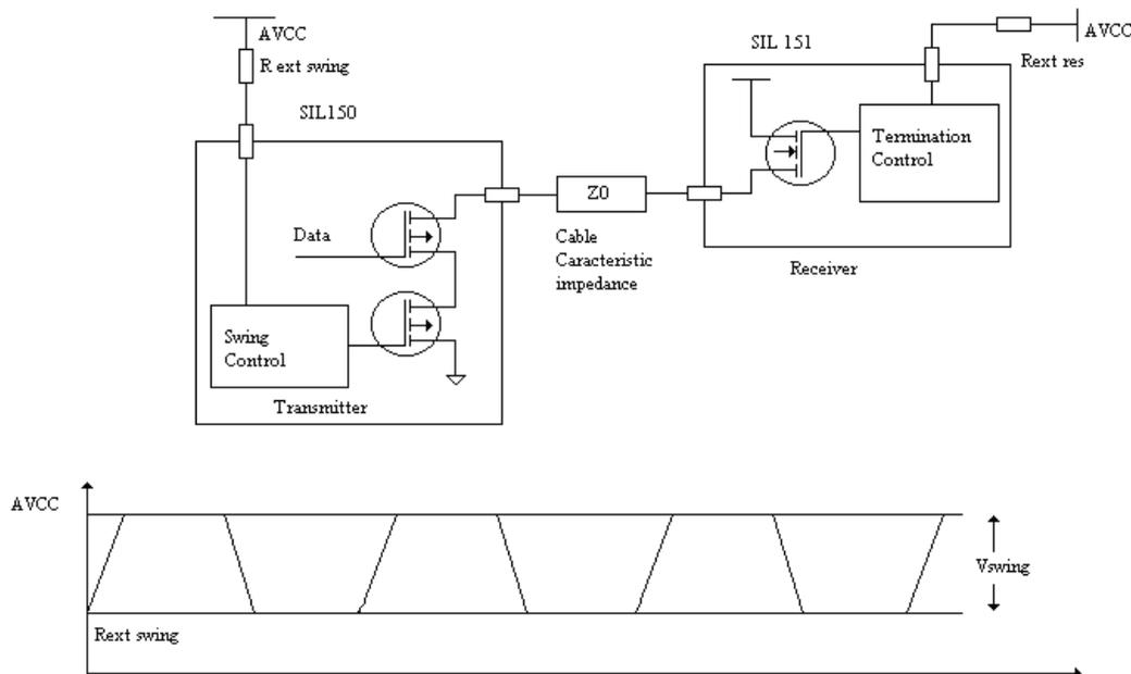
Fig2. Sil 150/151 differential signaling circuit
