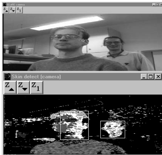
Fig. 2: example of a camera image. Top: grayscale image. Bottom: image of fully saturated colors, classified skin regions (white) and the two bounding boxes of skin-colored blobs (rectangles).
