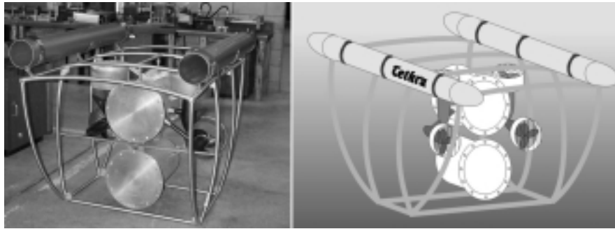
Figure 1 Photograph and computer aided drawing of the AUV.
