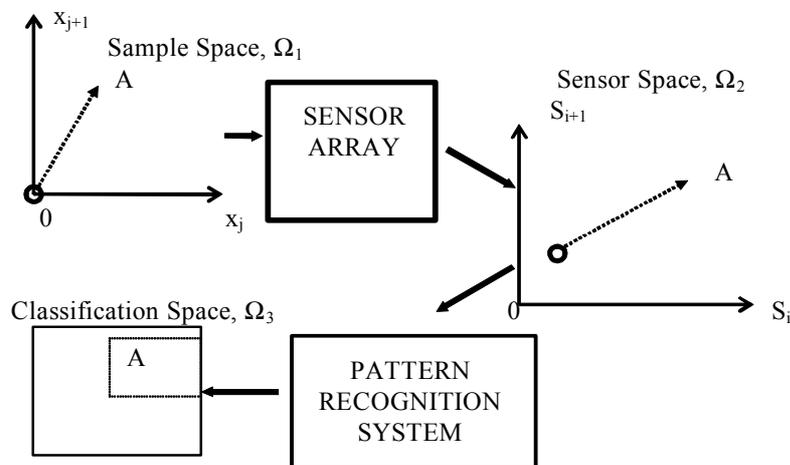
Fig. 5. Signal processing in an electronic nose.
