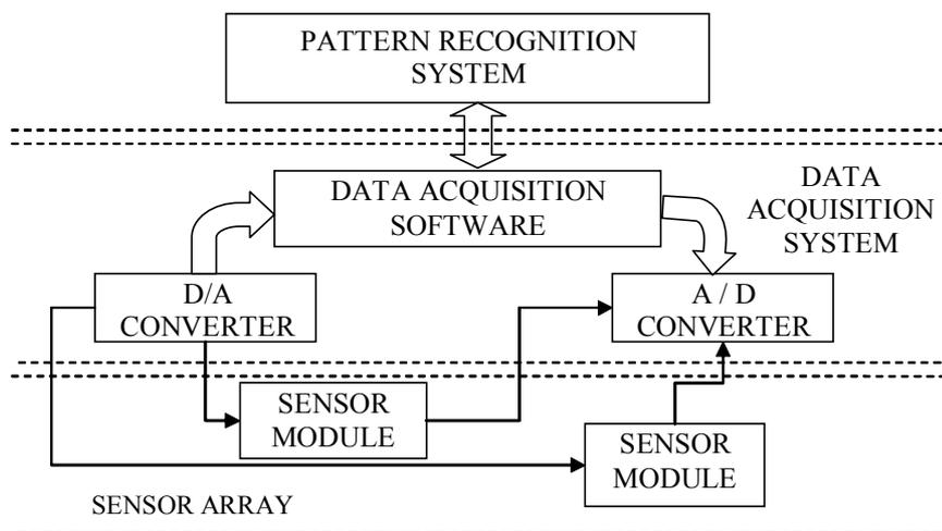
Fig.1. Block diagram of the electronic nose.
