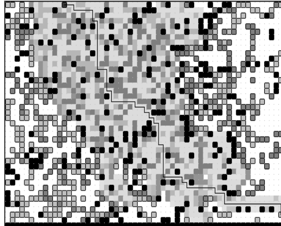
Figure 3. Results of D* algorithm: optimal path and cell expansion.
