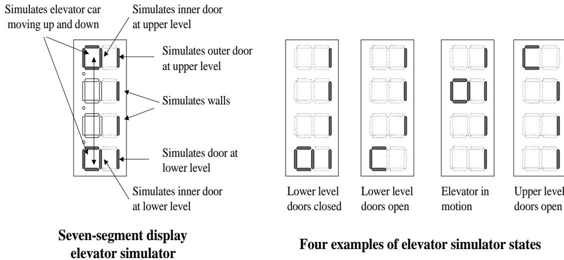
**Figure 1** Using the 7-segment display to represent the elevator.
