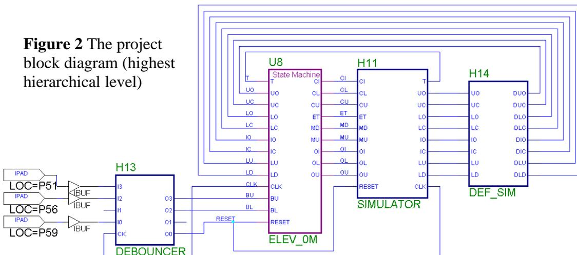
**Figure 2** The project block diagram (highest hierarchical level)
