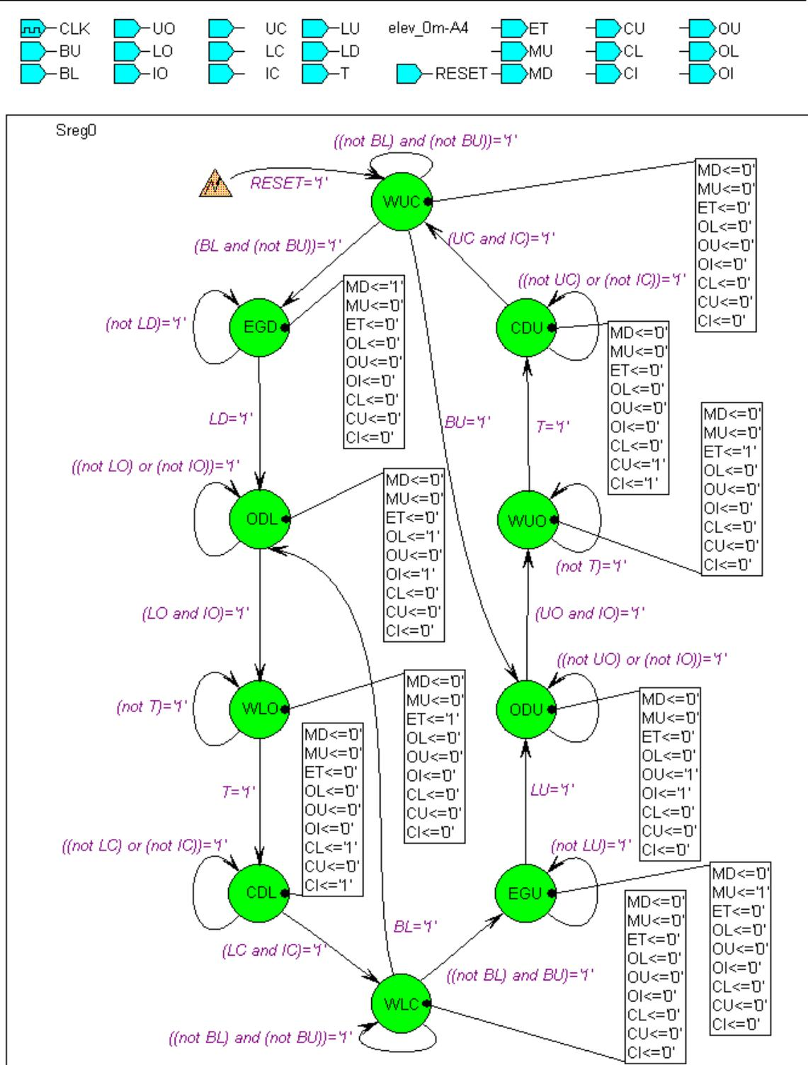
**Figure 3** The state diagram edited using the Xilinx Foundation Series State Editor.
