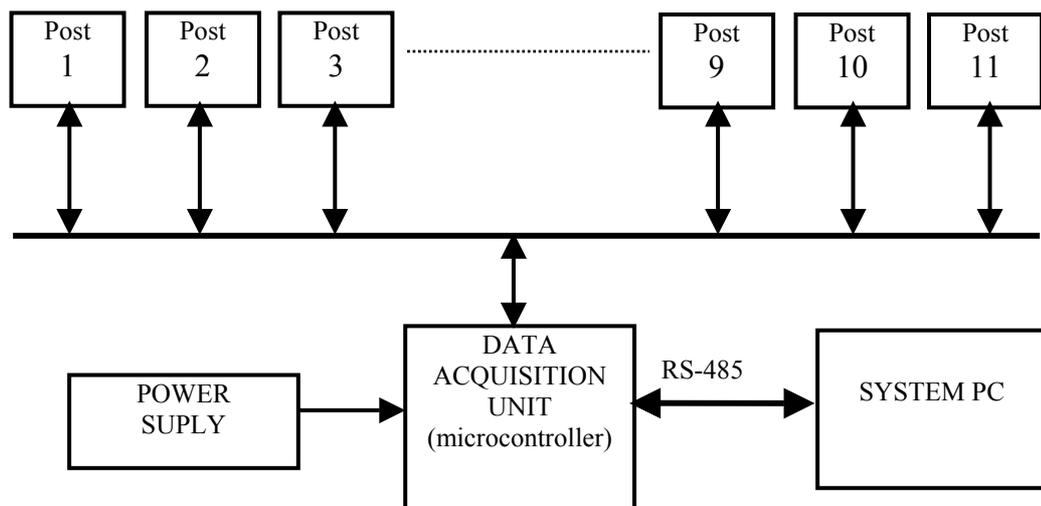
Fig. 1. The block scheme of monitoring system of spark plugs production.
