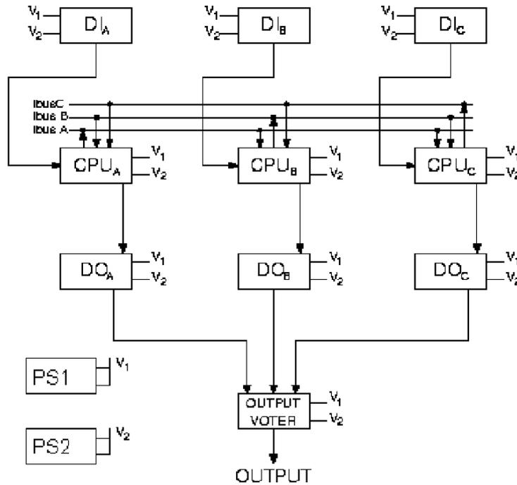
Figure 1. The PLC block diagram
