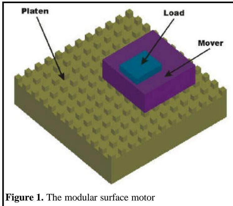
**Figure 1.** The modular surface motor
