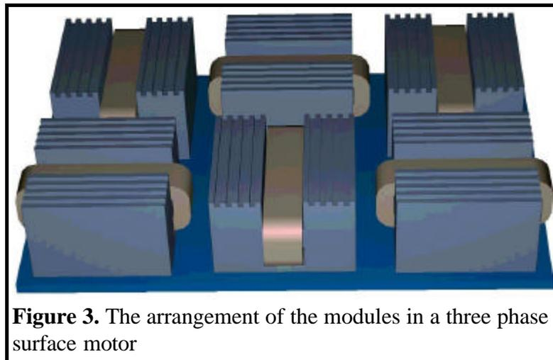
**Figure 3.** The arrangement of the modules in a three phase surface motor
