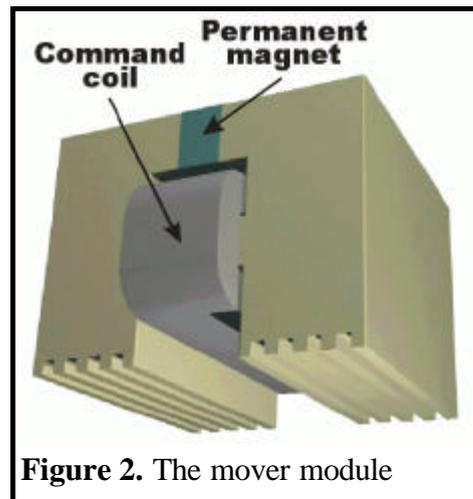
**Figure 2.** The mover module
